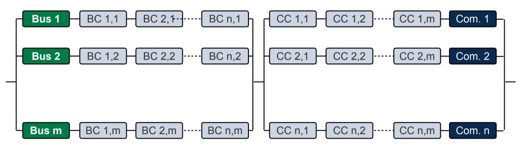
$$\begin{aligned} R_{whole}(n,m) &= \left(1 - \left(1 - R_{Bus} \cdot R_{BC}^{n}\right)^{m}\right) \cdot \left(1 - \left(1 - R_{Computer} \cdot R_{CC}^{m}\right)^{n}\right) \\ then: \ R_{CC}, R_{BC} &< 1: \lim_{n, m \to \infty} R(n,m) = ?? \end{aligned}$$
