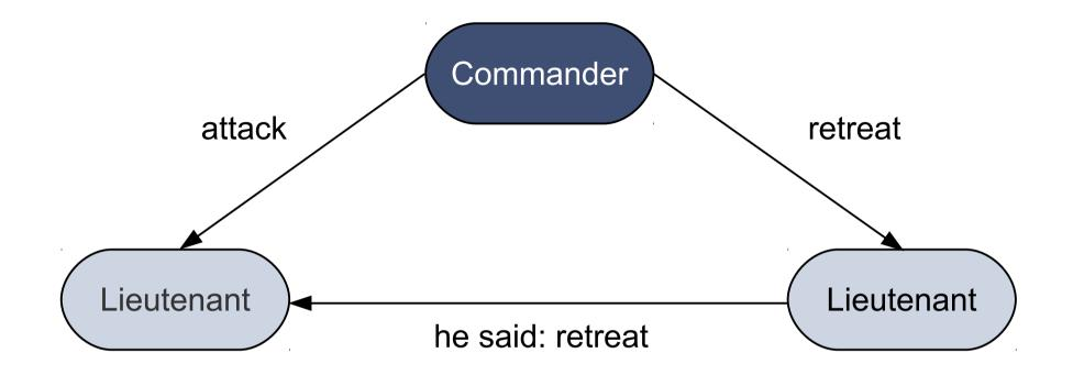
3 processes not sufficient to tolerate 1 traitor
