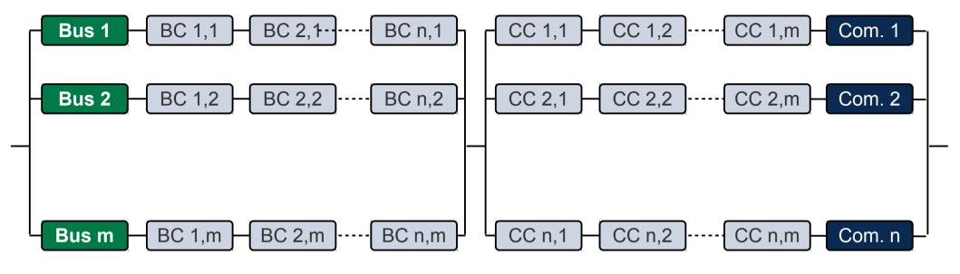
$$R_{whole}(n,m) = \left(1 - \left(1 - R_{Bus} \cdot R_{BC}^{n}\right)^{m}\right) \cdot \left(1 - \left(1 - R_{Computer} \cdot R_{CC}^{m}\right)^{n}\right)$$
