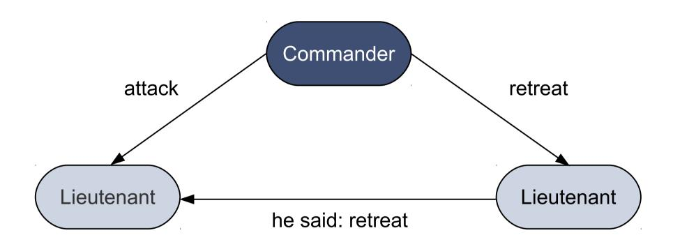
3 processes not sufficient to tolerate 1 traitor
