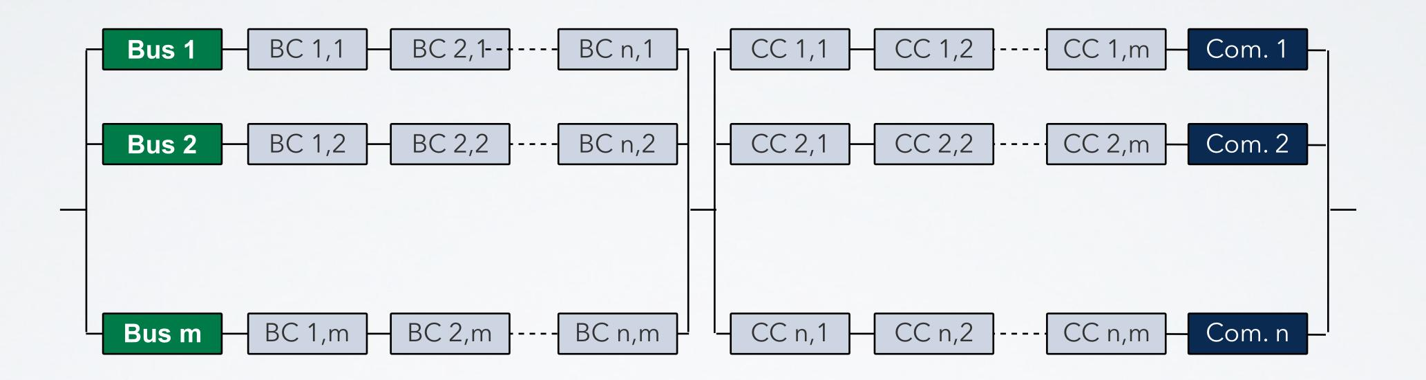
$$R_{whole}(n, m) = \left(1 - \left(1 - R_{Bus} \cdot R_{BC}^{n}\right)^{m}\right) \cdot \left(1 - \left(1 - R_{Computer} \cdot R_{CC}^{m}\right)^{n}\right)$$
