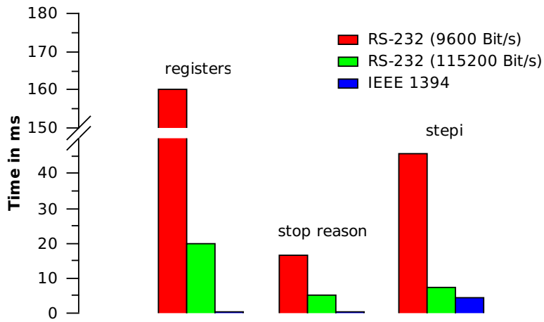
Figure 6.2: The amount of time needed for common debugging operations at the level of the GDB remote protocol. registers retrieves the contents of general-purpose registers. stop reason is used by the debugger to figure out why the target stopped. stepi steps a single instruction on the target system.
