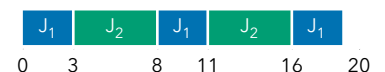
Figure 2: EDF produces a feasible schedule for the task set from Table 2. Between time units 19 and 20 the processor is idle.
