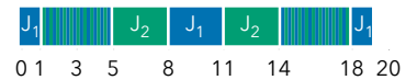
Figure 4: LST schedule with degradation to time-slicing between time units 1 to 5 and 14 to 18.
