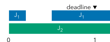
Figure 15: Deadline misses due to blocking and execution time overrun.
