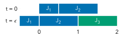
Figure 16: The release of J_3 causes overload. J_1 is 'pushed' into the past and will eventually be demoted to EDF Recovery.
