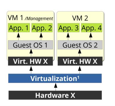
**Type-1 Hypervisors** provide virtual machines without the help of an operating system (directly on the hardware, bare-metal).
