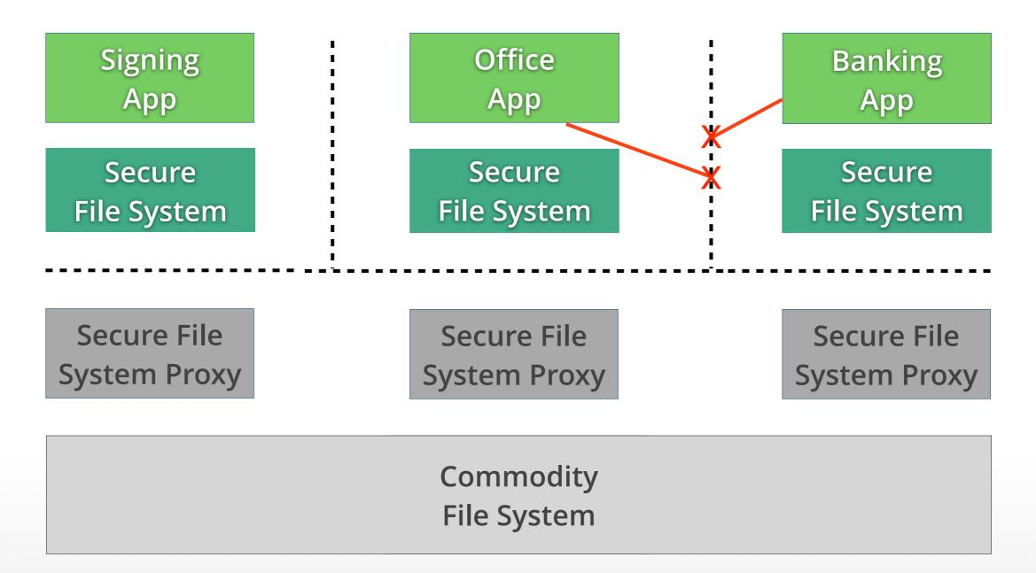
Isolate applications and their private storage: configure communication capabilities such that each application can access its private instance of the secure file system exclusively
