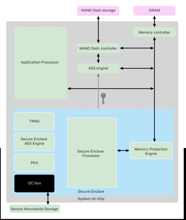
Apple devices have "Secure Enclave Processor (SEP)" running a dedicated service OS fully isolated from from the application processor hardware.
