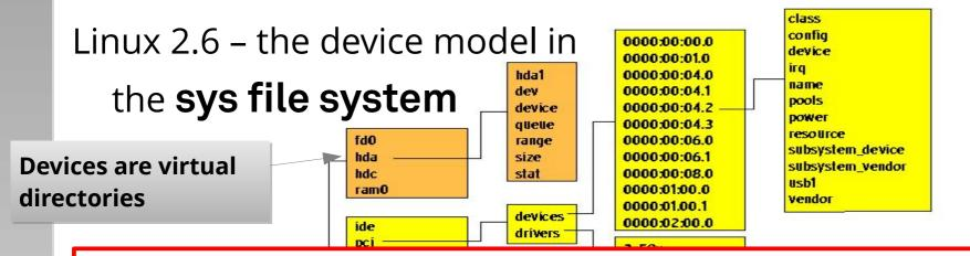
The device model allows kernel and applications to explore the available hardware. For example, power management can stop and restart dependent devices in the correct order.
