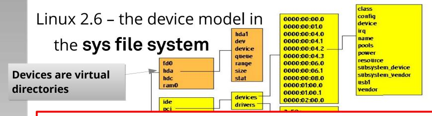
The device model allows kernel and applications to explore the available hardware. For example, power management can stop and restart dependent devices in the correct order.
