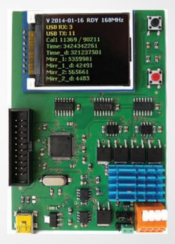
energy measurement resolution: 0.1uJ, temporal resolution 6ns (~150kHz)
