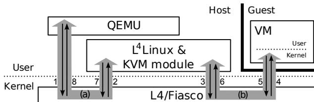
Figure 2: KVM-L4 control flow
