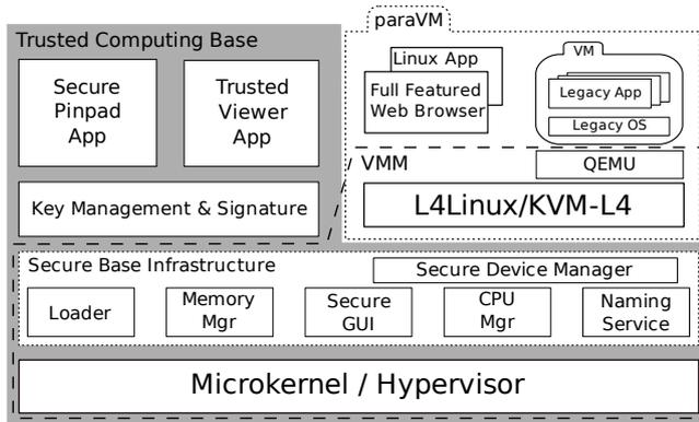
Figure 3: System Architecture.
