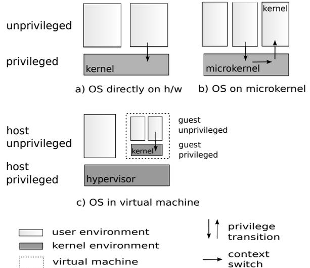
**FIGURE 1:** A system running directly on hardware, on top of a microkernel and inside a virtual machine.
